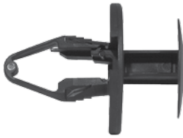
247-458 Std. Pkg. 25 pcs. Head Dia. 25mm, Stem Length: 20mm FORD 2005-on Fender, Flare, Gas Tank & Panel Attach. Push-Type Retainer Fits into 10.5mm Hole, Panel Range: 3.0mm-6.0mm #W712665-S300 CL Part No: 910-0651, Pieces: 2
