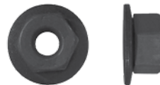
244-953 Std. Pkg. 25 pcs. M5-0.8 FORD Washer Nut 15 mm Washer O.D., Hex Size: 10mm, Height: 7mm #N621903
