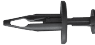
247-404 Std. Pkg. 25 pcs. Head Dia. 11/16", Stem Length: 7/8" GM 1984-on Exterior Body Panel Retainer Fits into 9/32" Hole #20590899, 20452072 CL Part No: 910-0560, Pieces: 4
