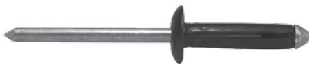
247-311 Std. Pkg. 25 pcs. Dia. 3/16", Flange Dia. 7/16" FORD, GM Black Split-Type Aluminum Rivet Grip: 5/64"-15/64" FORD #N805592-S100, GM #25618730 CL Part No: 910-1885, Pieces: 2
