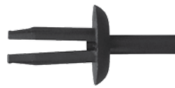
247-465 Std. Pkg. 25 pcs. Head Dia. 19/32", Stem Length: 5/8" FORD 1978-on Fender Sheild Retainer Fits into 1/4" Hole #387843-S CL Part No: 910-0790, Pieces: 4
