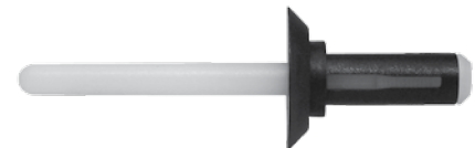
247-313 Std. Pkg. 25 pcs. Dia. 5/32", Flange Size: 11/32"x5/8" FORD AEROSTAR 1986-on Cowl Vent Grille Retainer Rivet Grip Range 5/64"-13/32" #N804583-S CL Part No: 910-1835, Pieces: 3
