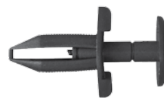
247-417 Std. Pkg. 25 pcs. Head Dia. 17mm, Stem Length: 16mm GM C&K Truck 1999-on Fender/Front Bumper Cover Retainer Fits into 6mm Hole #15149708 CL Part No: 910-0605, Pieces: 2
