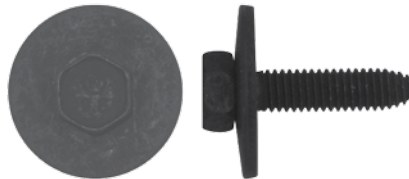
245-408 Std. Pkg. 25 pcs. M6-1.0x25mm GM Body Bolt Phosphate 24mm Washer O.D., Hex Size: 10mm #11503982 CL Part No: 910-0053, Pieces: 4
