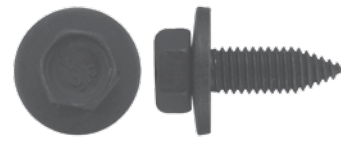
245-420 Std. Pkg. 25 pcs. M6.3-1.0x20mm GM Body Bolt Phosphate 17mm Washer O.D., Hex Size: 10mm #11501105 CL Part No: 910-0070, Pieces: 4
